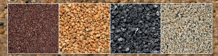
Elastopave can be used with crushed stone and gravel in many different colors and grain sizes. Stone sizes from ø 1.5 mm through to approx. Ø 10 mm are possible.
